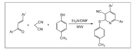
A series of 2-*p*-tolylthiopyridine derivatives was directly synthesized *via* three-component reactions of chalcones, malononitrile, and 4-methylbenzenethiol catalyzed by  $Et_3N$  in DMF under microwave irradiation. It is an efficient and promising synthetic strategy to construct 2-thiopyridine skeleton with the advantage of short time, excellent yield, and convenient operation.
